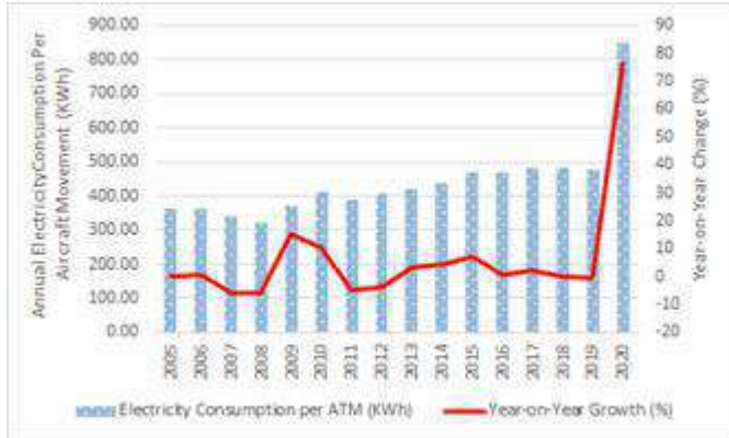
Fig.6: The annual electricity consumption per aircraft movement at Oslo Airport Gardermoen and year-on-year change (%): 2005-2020. Source: Data derived from Oslo Airport AS (2008, 2011, 2016, 2021).
