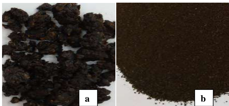
Fig. 1- Physical aspect of samples after mechanical treatment of cashew nut shells: (a) Grounded fresh shells; (b) old shells particles
