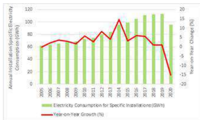
Fig.4: The annual electricity consumption for airport specific installations at Oslo Airport Gardermoen and year-on-year change (%): 2005-2020. Source: Data derived from Oslo Airport AS (2008, 2011, 2016, 2021).
