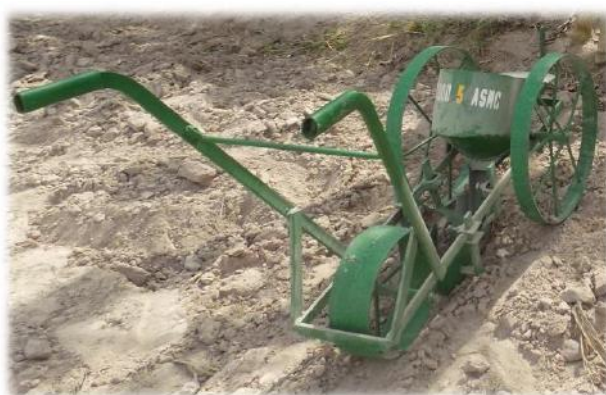
Fig.2: The ASMC seeder (Barro et al., 2022).
